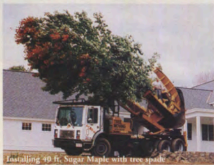
Installing 40 ft. Sugar Maple with tree spade
