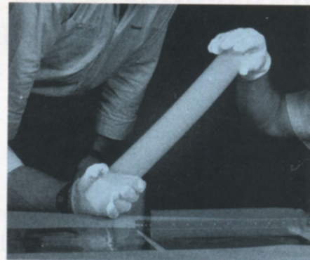
Only two to three times heavier than air, ultra-low density silica aerogel is the lightest known transparent solid; these pieces of the gossamer-like material come from the Lawrence Livermore National Laboratory.
