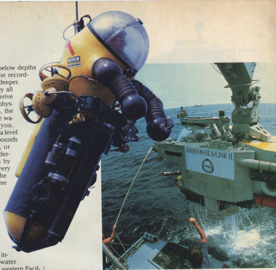
Rising from the depths, the Johnson Sea Link II is hoisted onto a recovery ship (above). Divers can enter and leave the JSL II while underwater. Wasp (left), worn by designer Hawkes, was the first suit to use thrusters, not human power.
