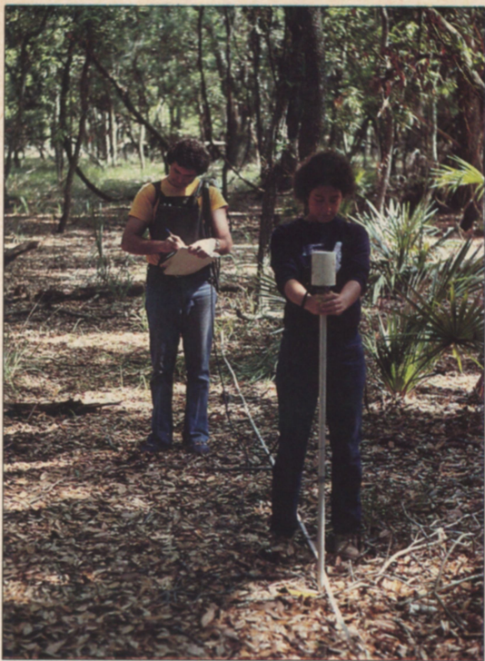
Following the plastic tape measure used to map the St. Catherines site, Deborah Mayer directs the sensor while Ervan Garrison records the magnetometer's readings (left). Their results helped locate the ancient site (right).
