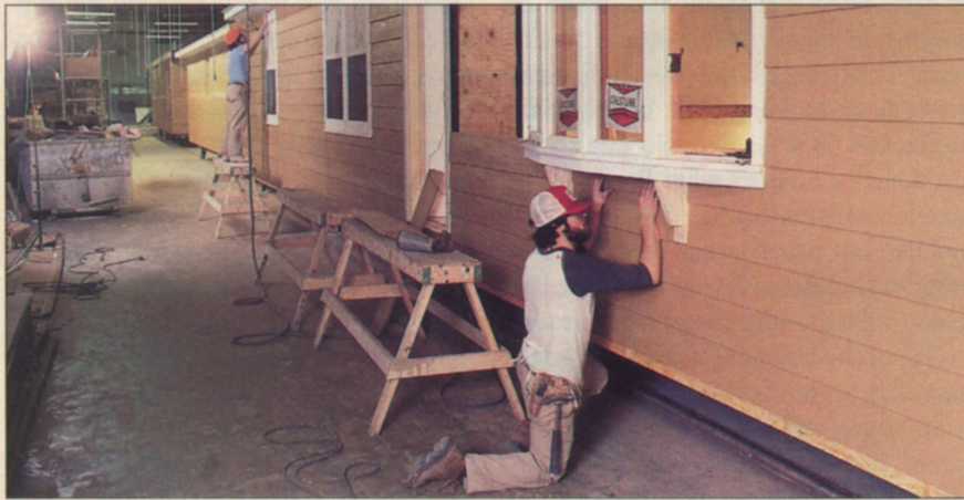
ABOVE: The houses-to-be move down the assembly line in various stages of completion. FAR RIGHT: In the first step of construction, the floor joists are built using a pneumatic nail gun. Once insulation has been attached (above right), siding is nailed into place (left). RIGHT: A grand vision of manufactured housing built for Montreal's Expo 67, Moshe Safdie's Habitat featured modular houses stacked like building blocks.
