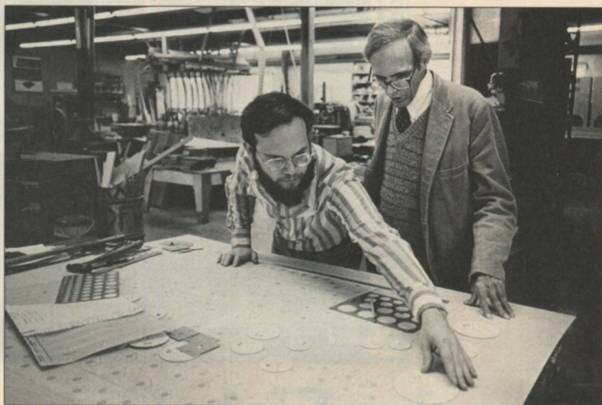
Left: Antique and new aluminum trackers rest on an 18th-century engraving. Below left: Metal disks (templates), stacked on spindles, are traced for pipe diameters when the wind chest is designed, as Fisk and his son Josiah are doing below. At right: Hand-pumped bellows like this one powered organs before electric blowers were introduced.
