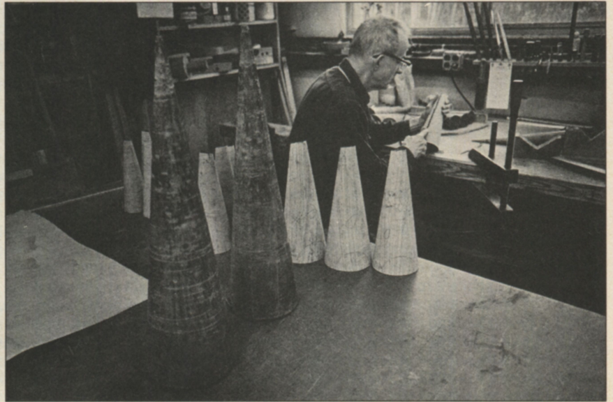
Left: A close-up of the mouths of a row of completed pipes. Below left: Using a portable drill press on the wind chest, Mark Clark drills holes that will lead to the ends of the pipes. Below: After pounding a lead sheet around a wooden form similar to those in front, David Gifford now prepares the seam of the pipe for soldering.
