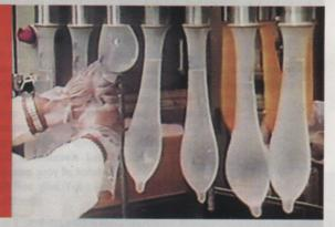
With individual electronic testing, every condom is checked for pinholes via an electrical switching system. All those that fail are discarded; the rest are sold.
